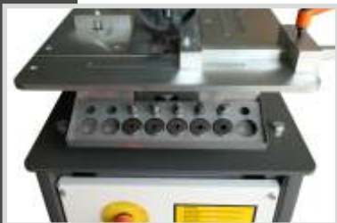
Standard set of punches included Ø 5, 6, 7, 8, 9 en 10 mm
