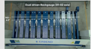
Dual driven Backgauge (X1-X2 axis)
